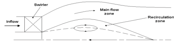
Fig. 2. Recirculation zone in swirling flow [7]
