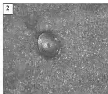
Fig. 2. Stereoscopic photograph of a Cu-Mo coating laser-eroded at 20 W ( $\times 57$  magnification)
