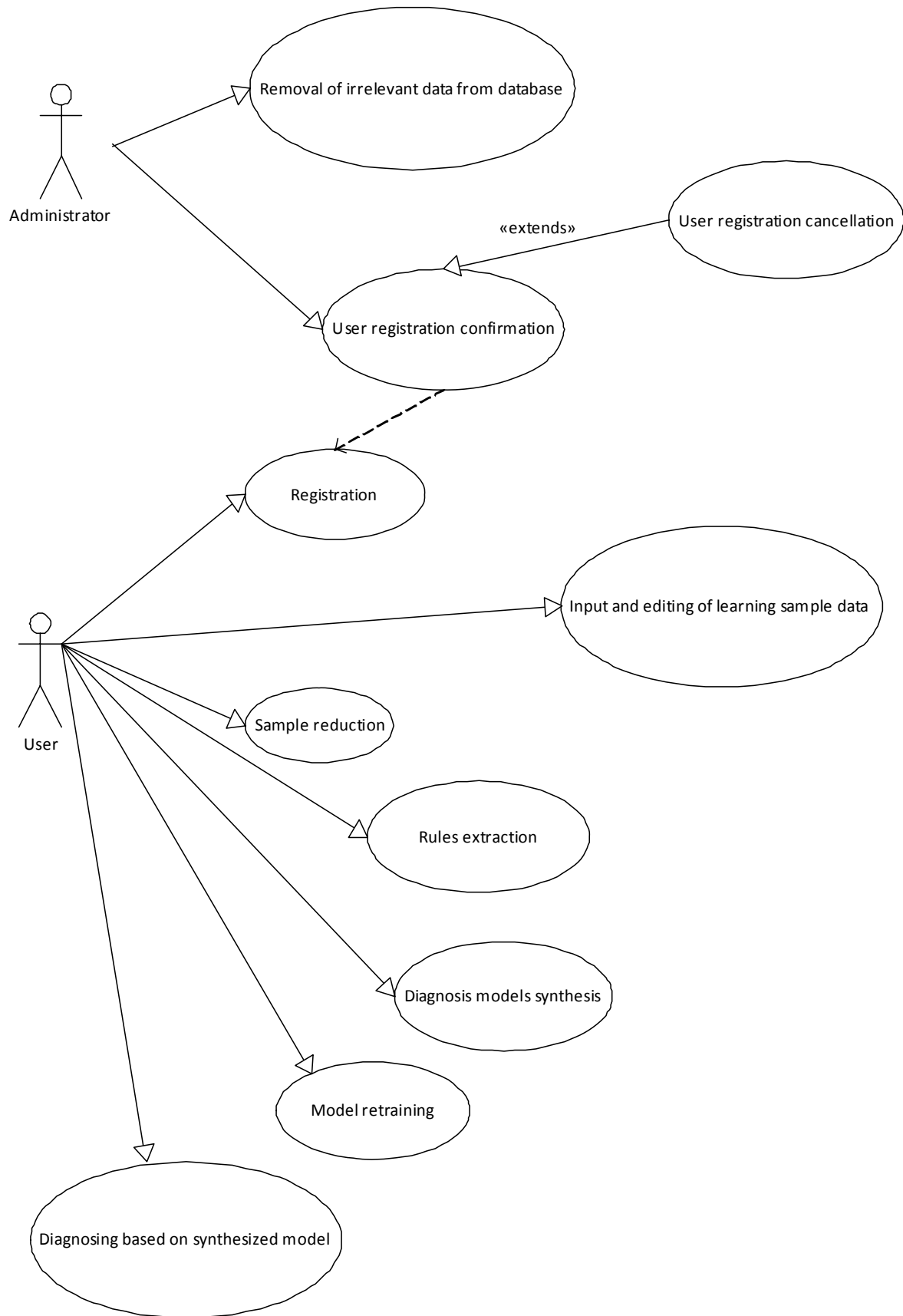
Figure 3 – Use case diagram of diagnosis models synthesis information technology
